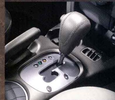
Dual-mode automatic transmission with SHIFTRONIC™ offers fully automatic or manual sport shifting 1 .
