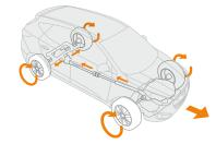
**ALL WHEEL GRIP** To help optimize traction when the going gets tricky, Tucson's available All Wheel Drive continuously varies the torque transfer between front and rear wheels automatically. Drivers can also select the 50/50 torque-split setting to balance power between front and rear wheels in snow or deep sand conditions.
