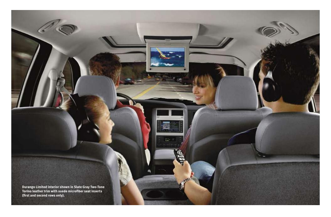
**REAR SEAT VIDEO**<sup>TM</sup> **SYSTEM.** This available system entertains rear passengers with a DVD player and a large eight-inch screen. This system also plays audio CDs and MP3 discs. A convenient jack allows for the connection of a video camera, a video game system, or MP3 player. A battery-powered remote control and two wireless headsets are included.
