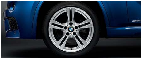
Double Spoke (Style 355M) 18-inch light alloy wheels. With run-flat 1 all-season tires 2 : 18 x 8.0 and 225/45 tires. With run-flat 1 performance tires 2,3 : 18 x 8.0 front, 18 x 9.0 rear and 225/45 front, 255/40 rear tires.
