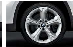
Star Spoke (Style 320) 18 x 8.0 light alloy wheels with 225/45 run-flat 1 all-season tires. 2
